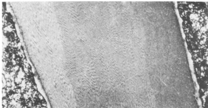
Figure 9 Sample no. 0020, insert type a, ternary Al-Ni-Cu eutectic, lower portion, viewed under polarized light, \theta = 20^\circ , longitudinal view, \times 65 .
