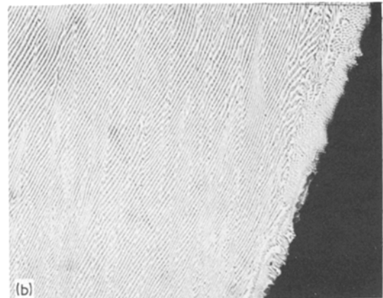
Figure 11. Insert type a, middle portion after the bend, downward face, depleted zone, longitudinal view, \times 65 . (a) Sample no. 0004, binary Al-Ni, \theta = 14^\circ . (b) Sample no. 0013, ternary Al-Ni-Cu, \theta = 14^\circ , corresponding schematic Fig. 12.
